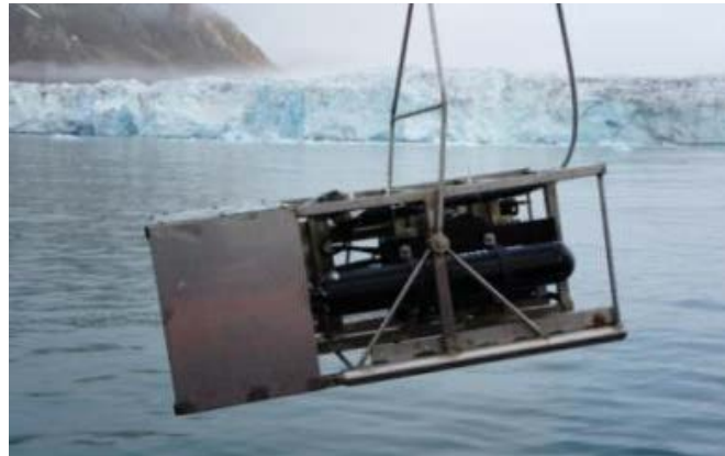
Laser Optical Plankton Counter (LOPC) - high-resolution automatic measurements of plankton biovolume spectra
