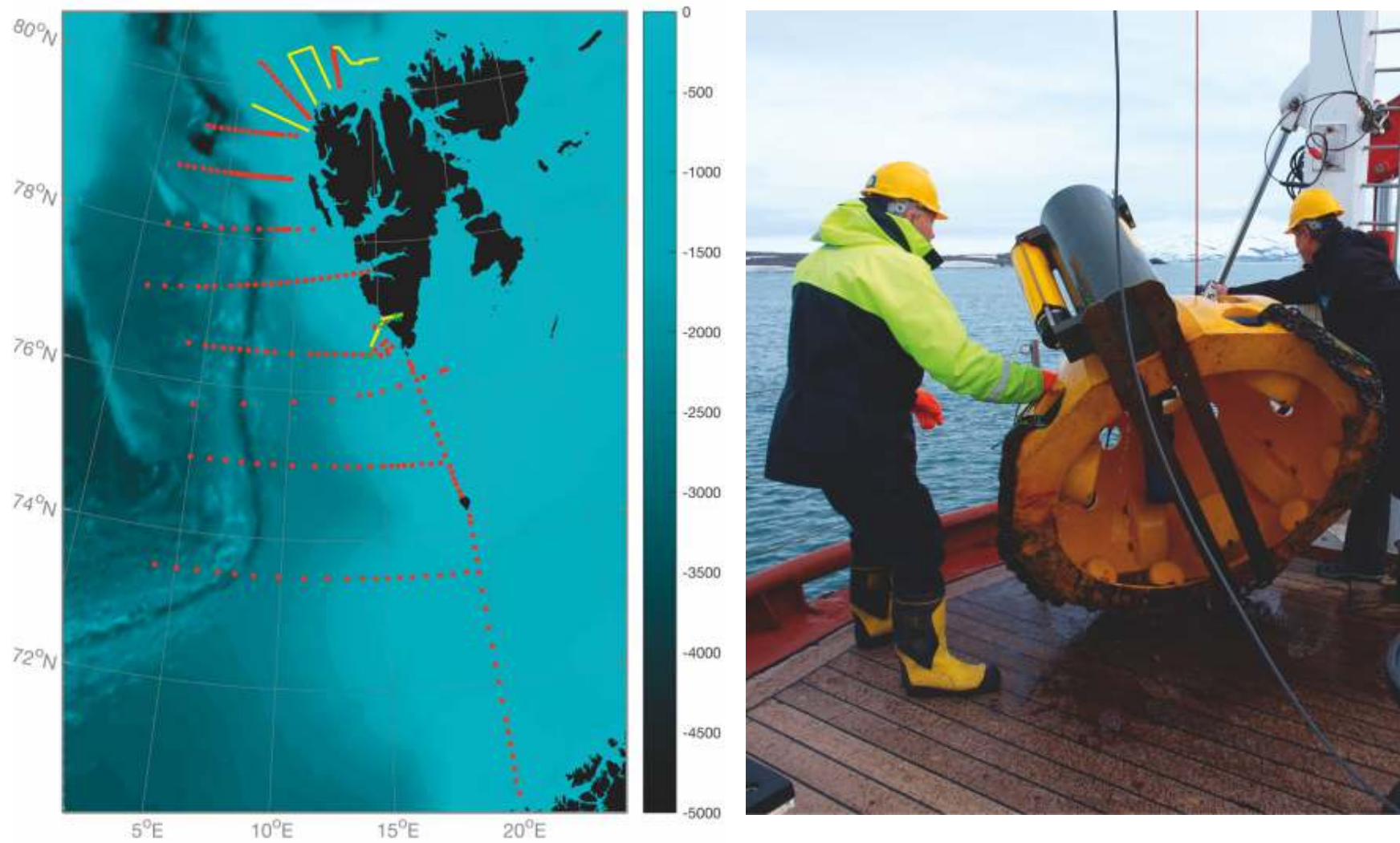
A map showing standard hydrographic stations (red dots) occupied by r/v Oceania during each summer survey and deployment of the bottom-mounted current meter in the fjord.
