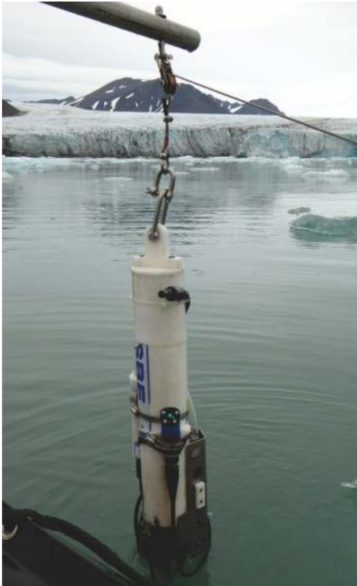
A conceptual model of ocean-air-ice interactions in the Hornsund area (upper right) and different instruments used for ocean, atmospheric and glaciological observations in the project – a CTD probe (left), an automated meteorological station (bottom middle), and a GPS station for monitoring glacier activity (bottom right).
